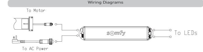
**Example 1:** Utilizing the Sunea<sup>®</sup> motor the receiver is plugged into the motor and both are powered from the same source via Sunea<sup>®</sup> power cord. The field installable motor plug allows the same configuration with other motors.
