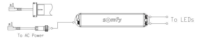
**Example 2:** The receiver and motor are plugged separately for power, each directly into the power outlet. NOTE: The receiver can be used with most 12V LED lights, up to 60w.
