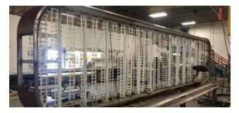
SignBOX II is recommended for installation 12" (300 mm) on center for depths of 5 - 6" (125 - 150 mm) from face, as this yields the same brightness as a fluorescent lit cabinet; however, in deeper cabinets at 8 - 9" (200 - 230 mm) from face, the spacing may be spread further to 14 - 16" (350 - 400 mm) on center, saving product, time, and money.
