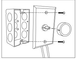
Mount dim control box assembly onto junction box. Attach knob onto shaft.
