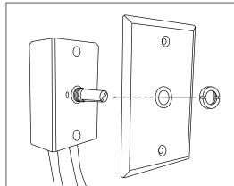
1. Mount switch plate to dim control box (P/N 701843) using round nut.
