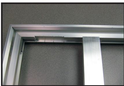
Notching the frame before assembly allows for the ability to change out Dividers or add new Dividers while in the field. Without notching the frame, the cabinet would need to be taken apart in order to make any changes to the Divider configurations.
