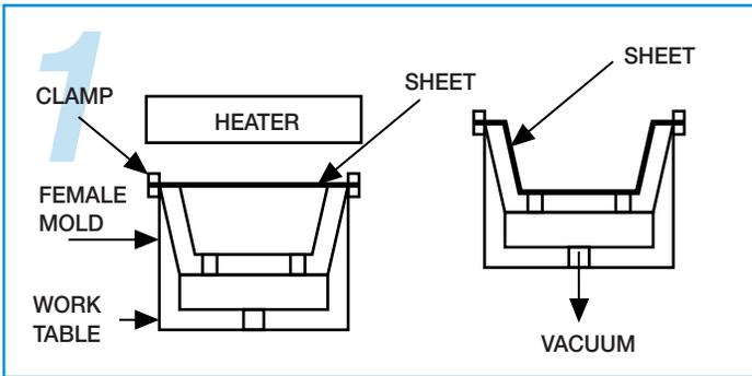
Straight vacuum forming in a female mold is recommended for low-profile parts where deep draw is not a requirement.
