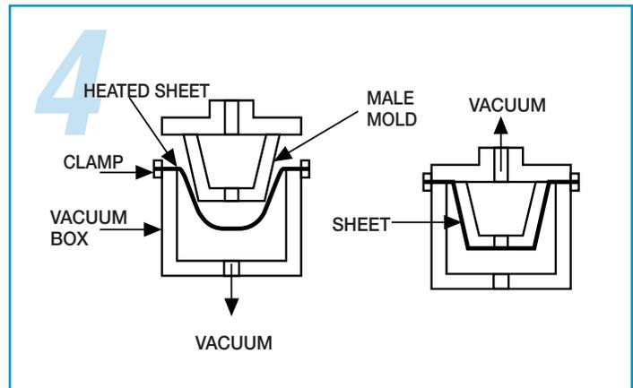
Vacuum forming with snap-back can reduce starting sheet size, aid material distribution, and minimize chill marks.
