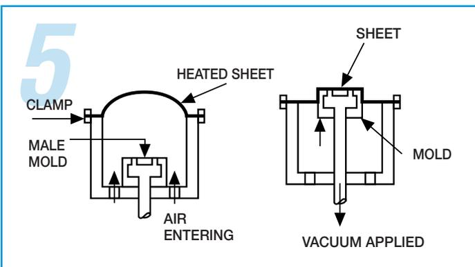
Air-slip forming is similar to vacuum snap-back except that heated sheet is billowed up and mold rises to meet it.
