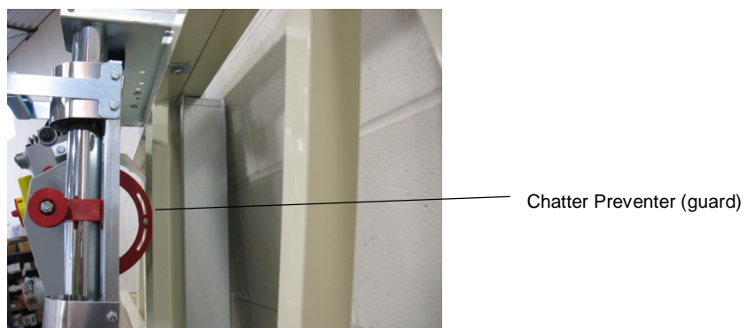
Figure 40: Chatter Preventer (guard) in position for crosscutting 6400 shown
