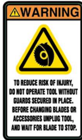
Do Not Use Without Blade Guard On Machine
