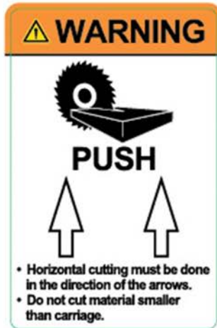
Feed Stock In The Direction Of The Arrow
