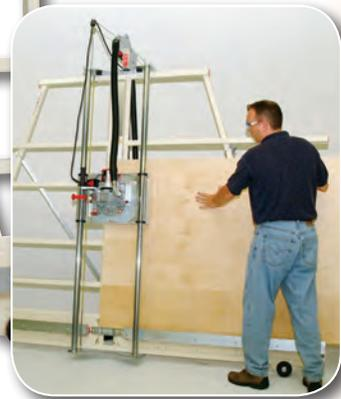
The popular H-Series saws are ideally suited for customers looking for a full sized vertical panel saw at a very affordable price. These saws are available in three crosscutting heights, 50", 64" and 74" while delivering an accuracy of 1/32" straight and square. With 3/4 Hp industrial motors, these versatile saws are used in a variety of panel cutting operations.
