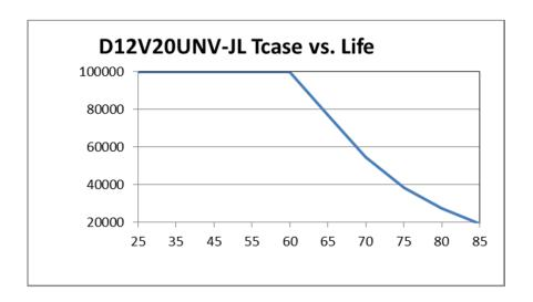
The Data curve provided predicts the LED Driver life based on the case temperature measured at the Tc location identified on the label or specification sheet. The Telecordia SR-332 standard is used to generate the prediction curves.
