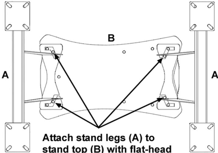
Attach stand legs (A) to stand top (B) with flat-head screws through these (4) holes
