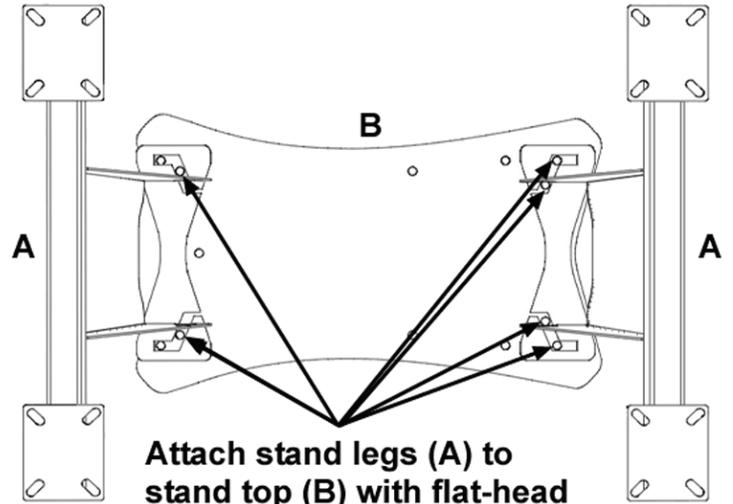
Attach stand legs (A) to stand top (B) with flat-head screws through these (6) holes
