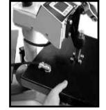
• Lift up on the heat platen slightly, enough to swing it out away from the bottom table. Lower the heat platen down and out of the clamp linkage.
