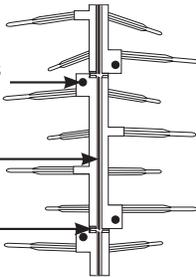
**NOTE: WHENEVER POSSIBLE, BIRD SPIKE STRIPS SHOULD BE SCREWED OR BOLTED DOWN IN CONJUNCTION WITH THE USE A NON-SILICONE OUTDOOR CONSTRUCTION-GRADE ADHESIVE.**
