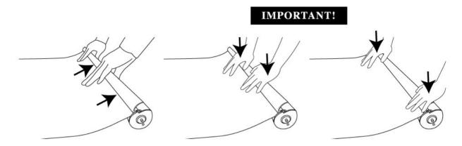
6. Return the roller with graphic into the base. Let the entire graphic lay outside the base. Close the cover.
